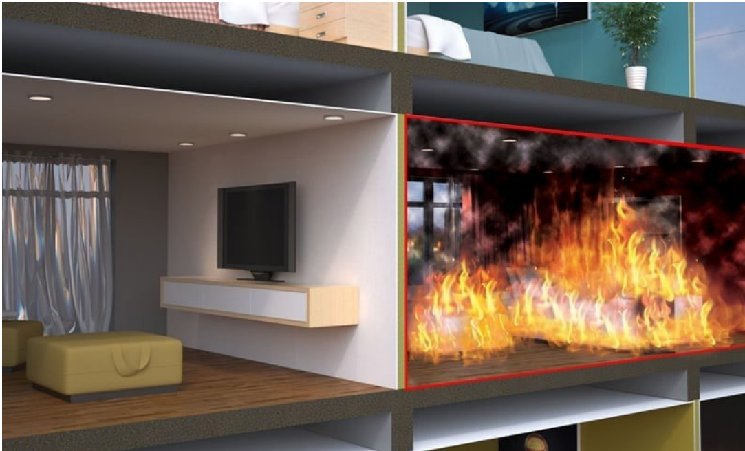
Figure 1 Compartment walls and floors between dwellings
