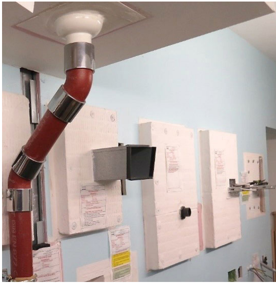
Figure 31 A sample of a penetration seal system
